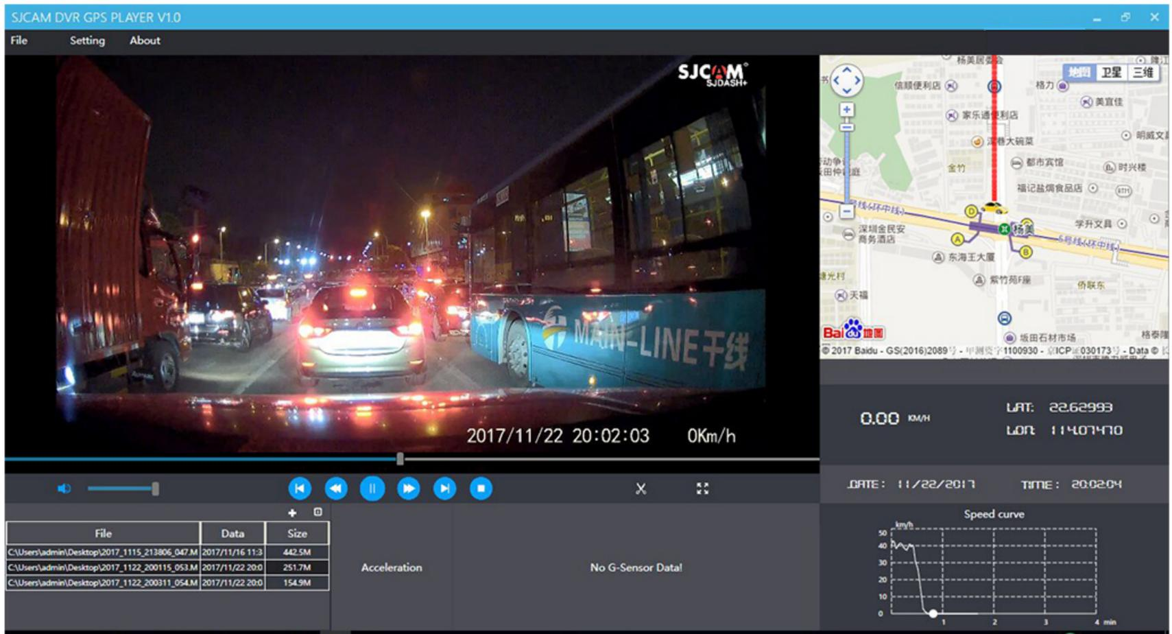
The main interface is a video, below is the file list. While the top right corner is the GPS map, and the software will display GPS Speed , time and some other information at the lower right corner.
